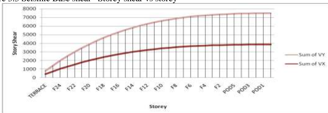
Figure 3.3 Seismic Base shear –Storey shear vs storey
